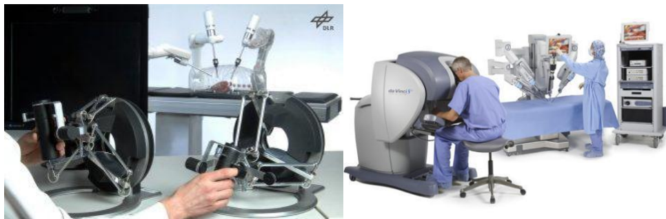
Figure 2: (Left) MIRO surgical robot from DLR controlled by Force Dimension's omega.7 haptic device (Right) da Vinci surgery system.
